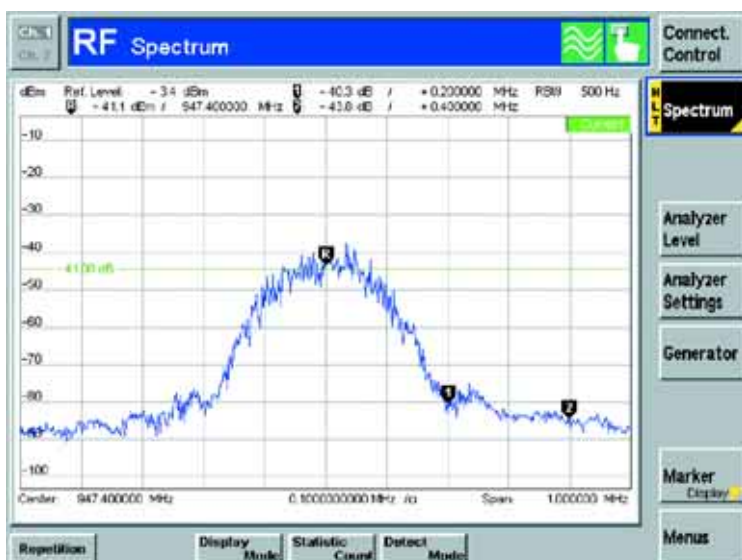
The spectrum analyzer provides several marker functions for a comprehensive investigation of the signal applied
